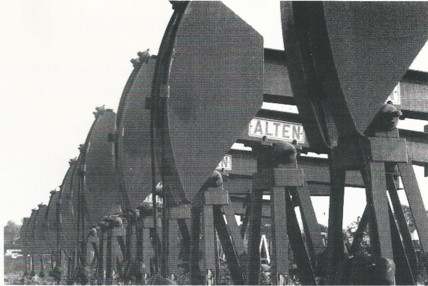
A row of Alten 16-43F-30P, Wide Base, Beam Balanced Units
