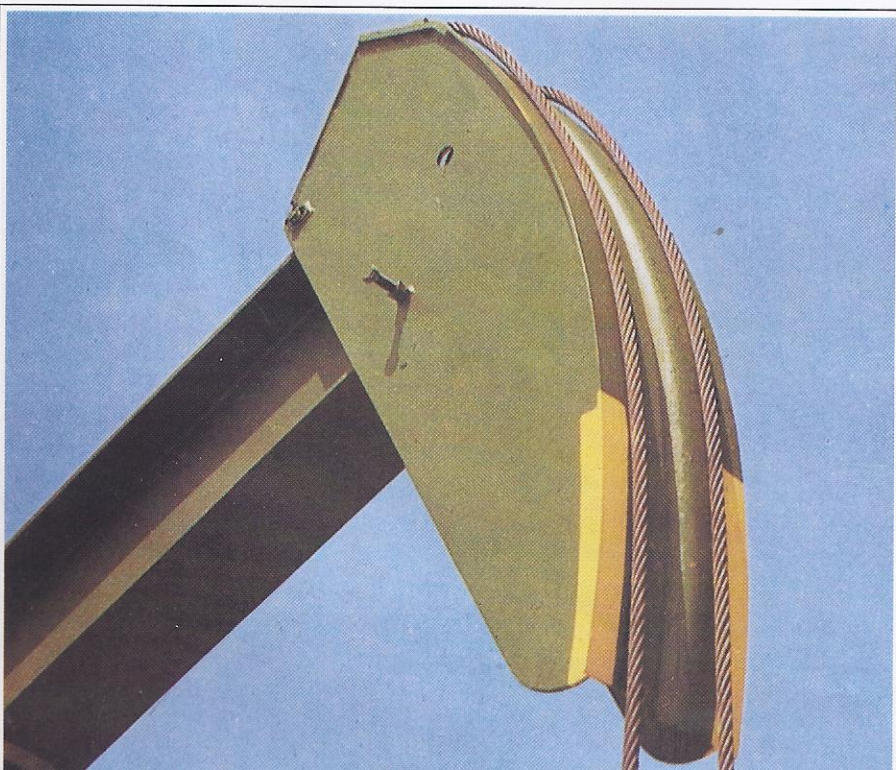
Horsehead and wire line assembly.
