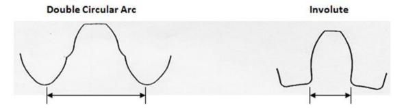
The wide tooth base results in lower tooth root bending stress than with involute teeth, resulting in greater bending strength torque. These features contribute to the excess torque capacity of DCA gear reducers.
