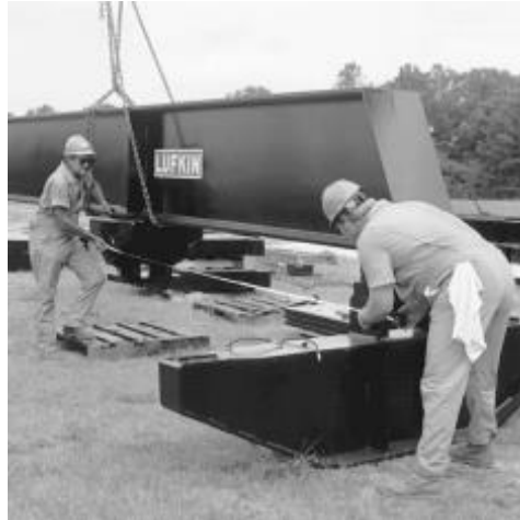
Figure 38: Verifying Center Bearing to Equalizer Bearing distance is equal on right and left side
