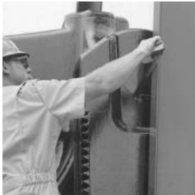
Figure 45: Measuring the distance between the pitman and the crankshaft
