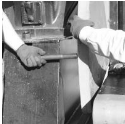
Figure 24: Auxiliary counterweight installation
