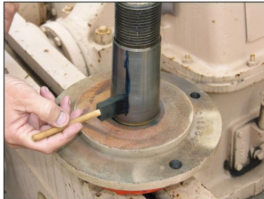
Figure 16: Application of machinist blue to check fit between pin and crank.
