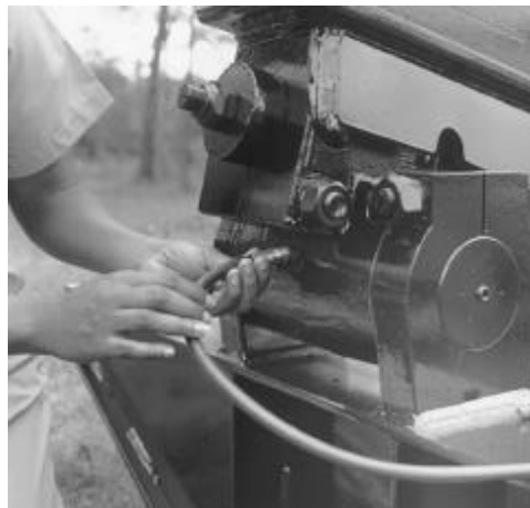
Figure 41: Equalizer Pin Lubrication
