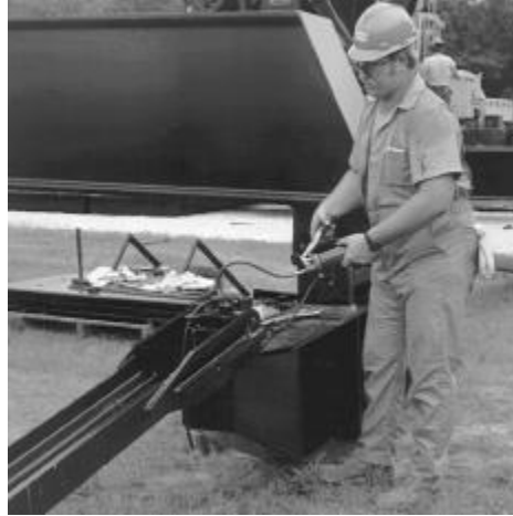
Figure 42: Lubricating the Pitman Box
