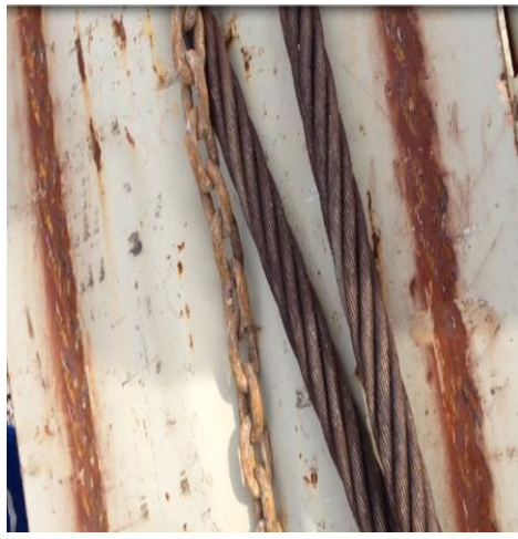
Horsehead with wireline removed. Wide tracking marks observed.
