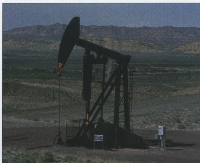
A Lufkin Air Balanced Unit with electric motor drive.
