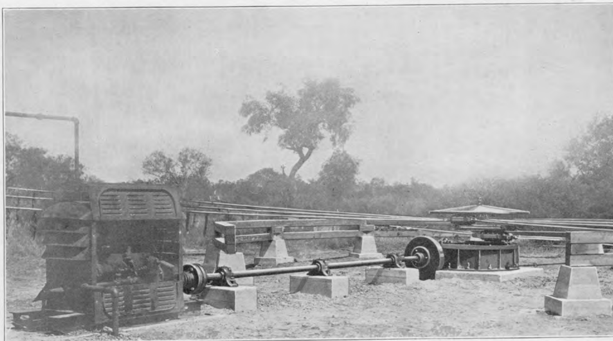
Allows straight connections to wells in any direction except very small angle space occupied by engine.
