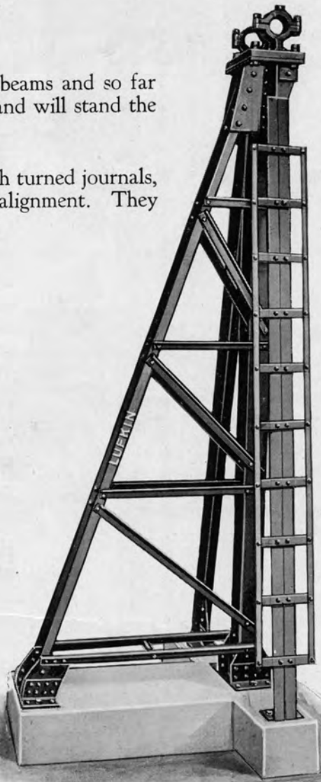
Standard I Beam Type Walking Beam (20" I Beam with 10" Channels) carried in stock; 14' Working Centers.
