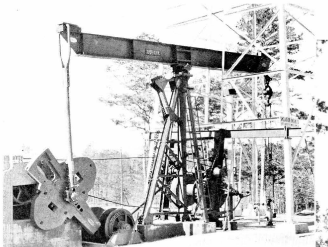
Sinclair Oil & Refining Co. Daisy-Bradford No. 2. Lufkin 6 1/2" H. B. Unit, Post Assembly and Hoist.
