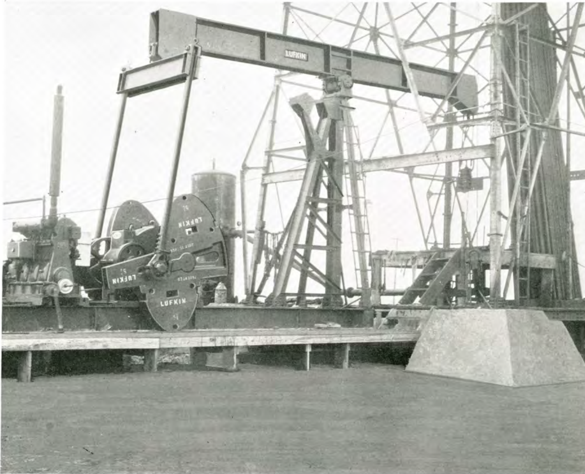
Lufkin Twin Crank Unit Assembly No. 0-A-58. Oklahoma City field installation.
