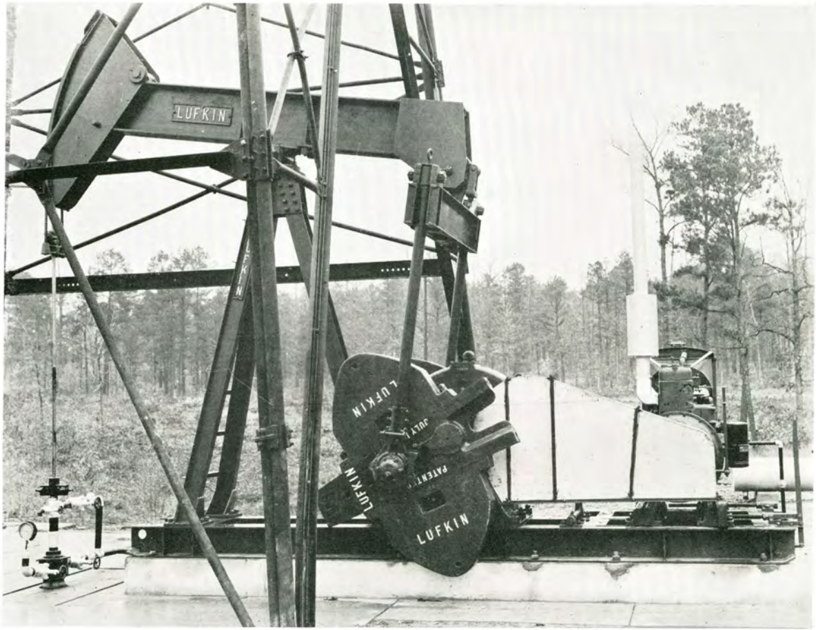
FIGURE 17 Lufkin Twin Crank Unit Assembly No. 3—20 to 30 H.P.—17,000 lb. Polish Rod Load, 54' stroke. See specifications page 843 and Blue Print below.
