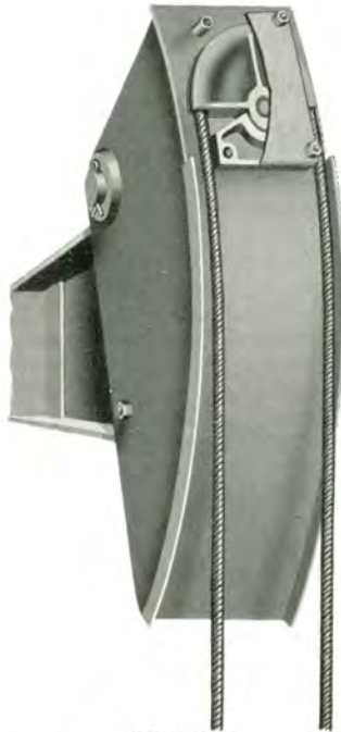
FIGURE 51 Hinged Horse Head showing Equalizer
