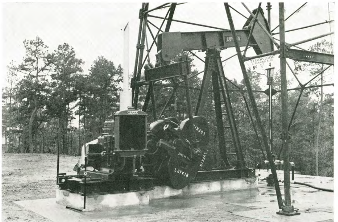
Lufkin Twin Crank Unit Assembly No. 3-18. Hundreds of these units are now in satisfac- tory operation.
