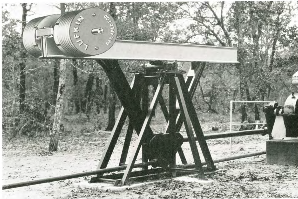
FIGURE 79 Lufkin Jack Type Take-Off with Rolling Counterbalance
