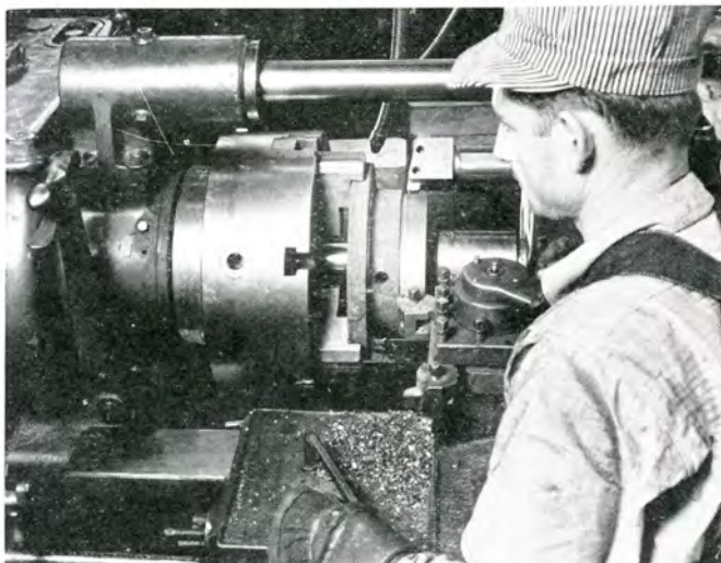
The most modern type of turret lathe—one of a battery performing similar operations. Note that boring, facing and turning rough and finish cuts are completed in one operation.
