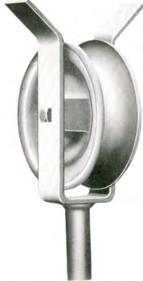
FIGURE 85—Lufkin 10" supporting sheave for 2½" pipe, commonly used with back crank take-off. The shank is made for 2" pipe and the sheave has a paraffined maple bushing.
