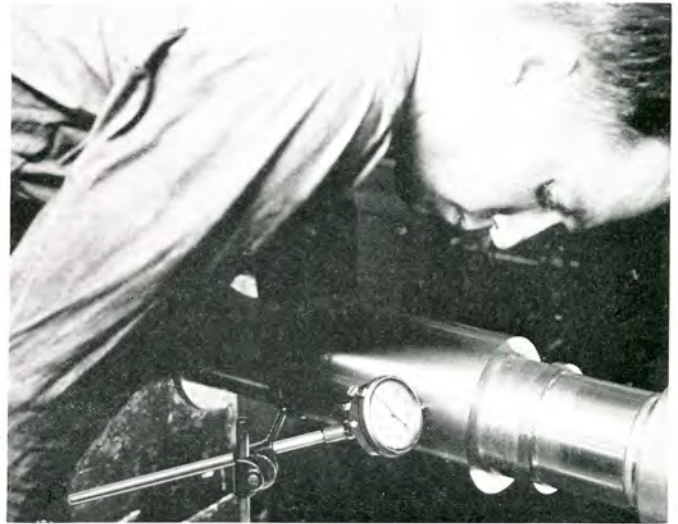
Testing pinion shaft blank for eccentricity before cutting herringbone teeth. Accuracy here is of extreme importance.
