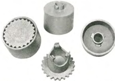
Heat Resisting Iron Gas Burner Casting
