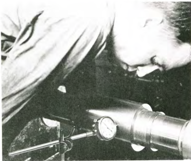
Testing pinion shaft blank for eccentricity before cutting herringbone teeth. Accuracy here is of extreme importance.
