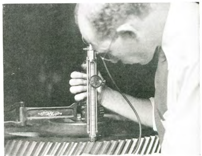
Testing gear teeth for hardness.
