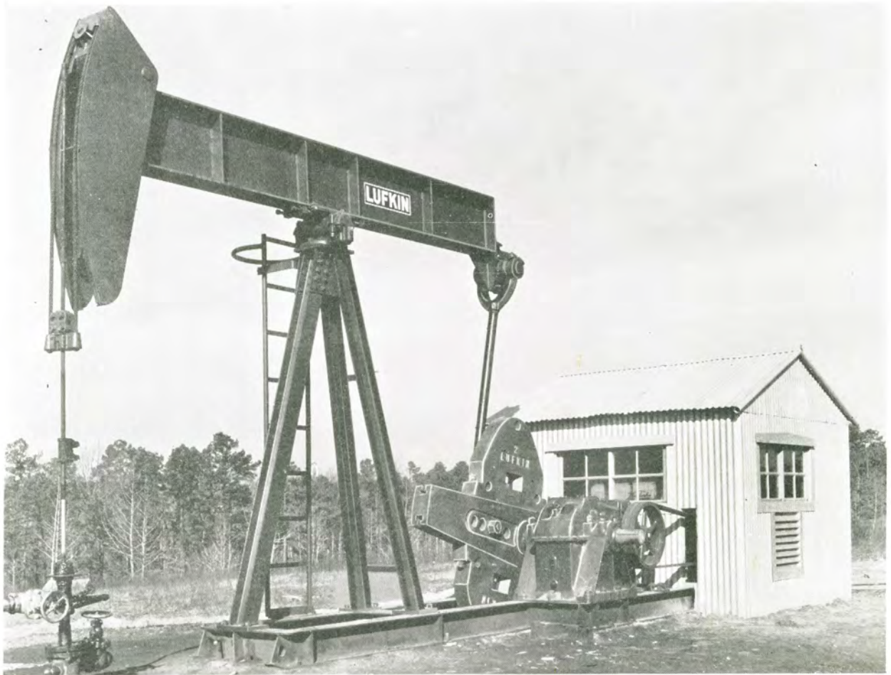
Bottom: Similar installation of heavier type with Universal Hanger and double channel single arm take-off pumping two additional wells.
