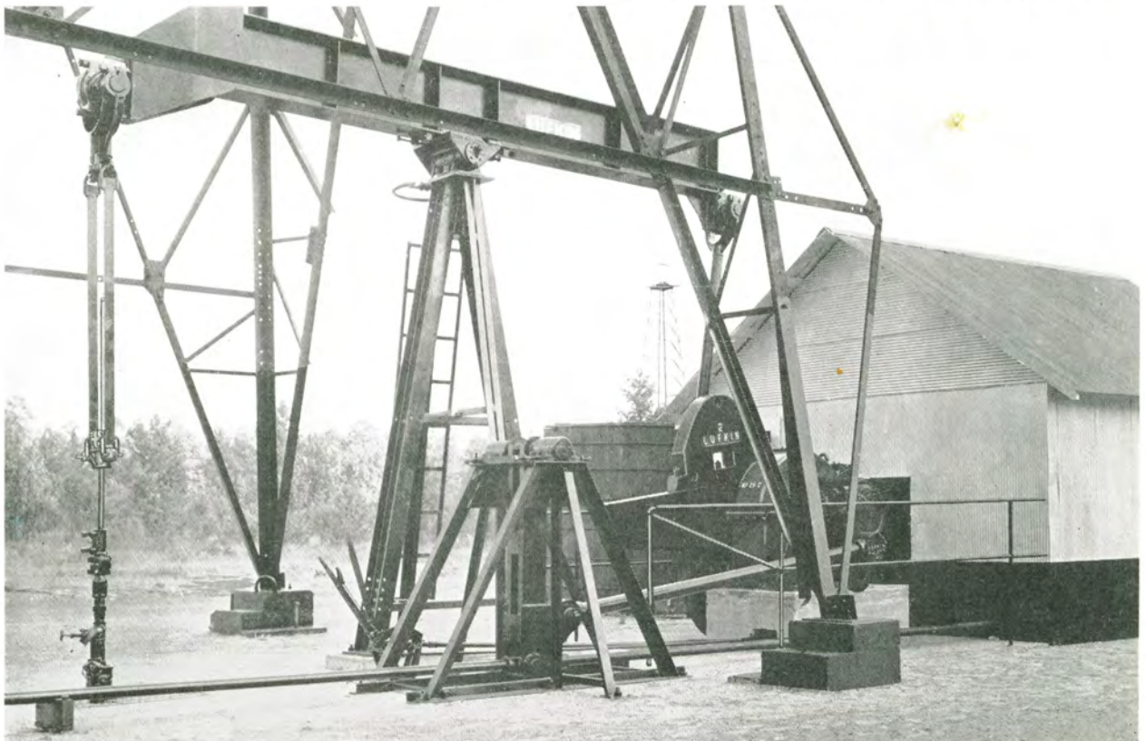
Bottom: Similar installation of heavier type with Universal Hanger and double channel single arm take-off pumping two additional wells.
