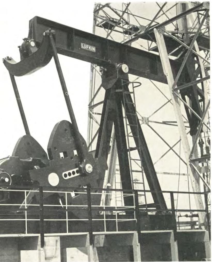
FIGURE 7 Lufkin "Universal" Units have all working points on the center line.
