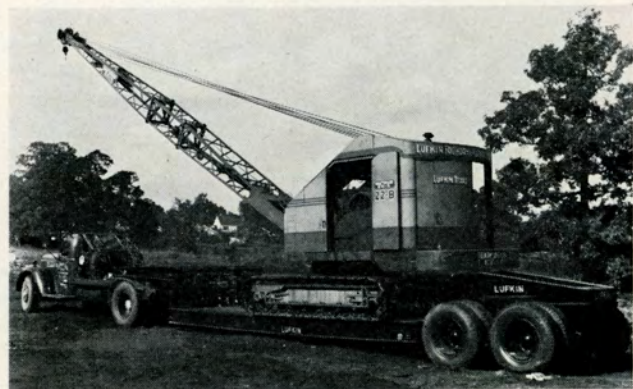
FIGURE 66 "Ready to Ride." This heavy machinery hauler may be loaded in ten to thirty minutes.
