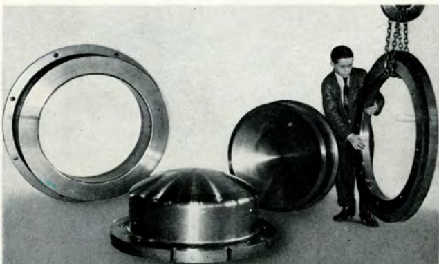
FIGURE 67 Die castings made of special alloy for presses up to 5000 tons capacity.
