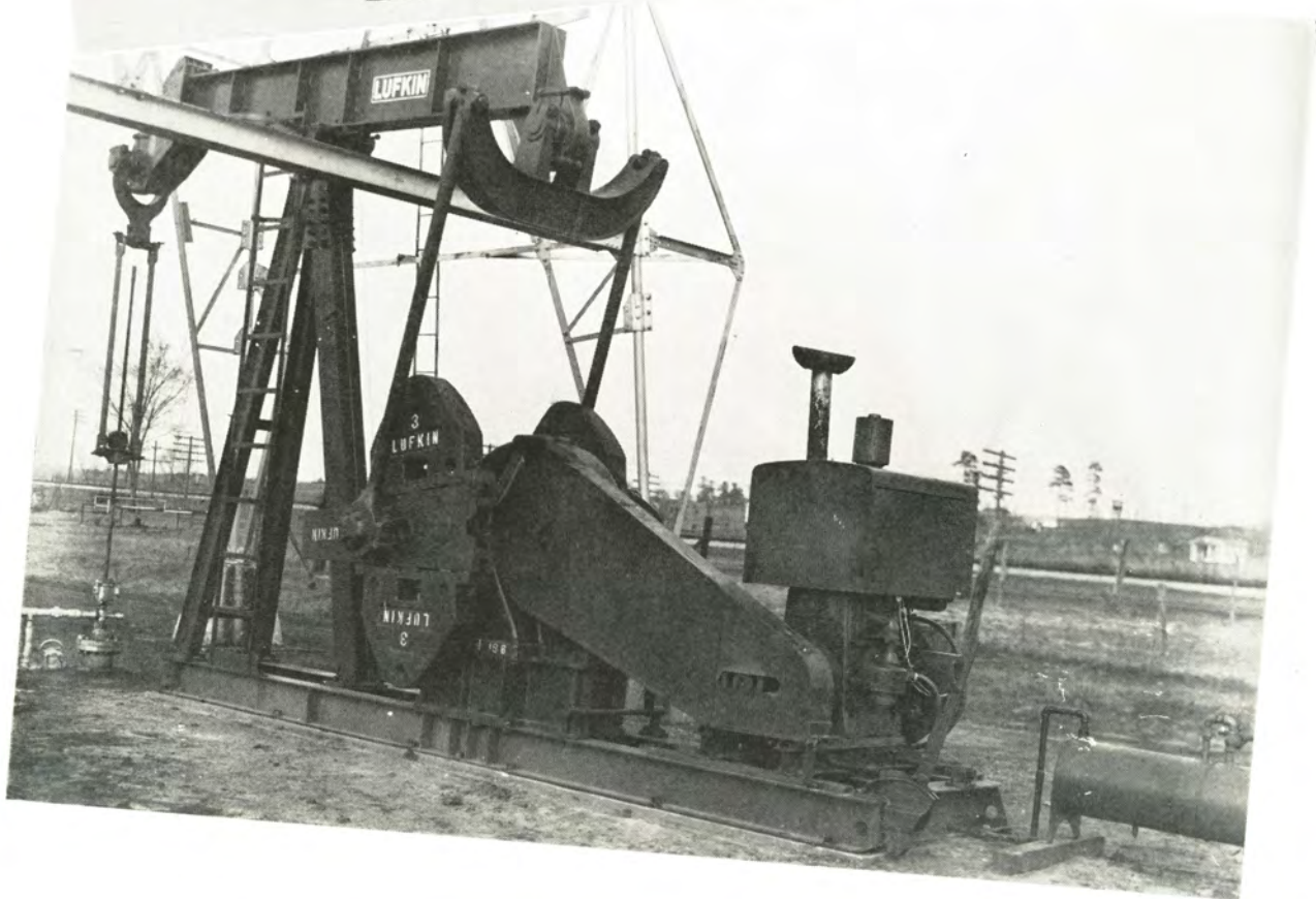
Above—Lufkin TC-OA-60A pumping unit with GSDH Lufkin-Cooper-Bessemer Horizontal Gas Engine Below—Lufkin TC-33A-18B pumping unit with Sub-base and GSC Lufkin-Cooper-Bessemer Vertical Gas Engine
