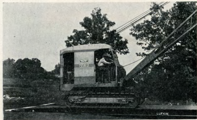
FIGURE 64 Nose Goose Neck folded down to ground level for loading.
