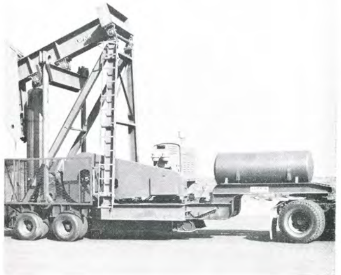
FIGURE 44 Mobile A-456D-120-36 Air Balanced Unit, Multi-Cylinder Engine Drive. This trailer-mounted unit with prime mover and diesel fuel tank built integral is ideal for test purposes.
