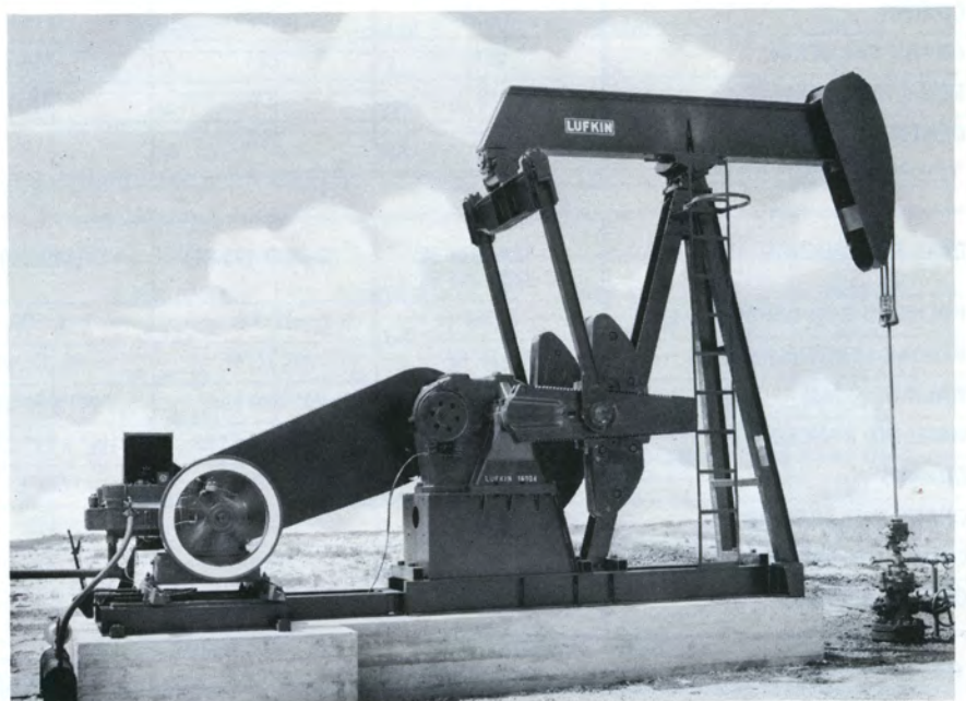
FIGURE 15 JOINTED ELL BASE adapts easily to all multi-cylinder engines by using slide rails. This type engine base can also be used with flywheel-clearing slow speed engines as shown on this C-160D-173-74 unit.
