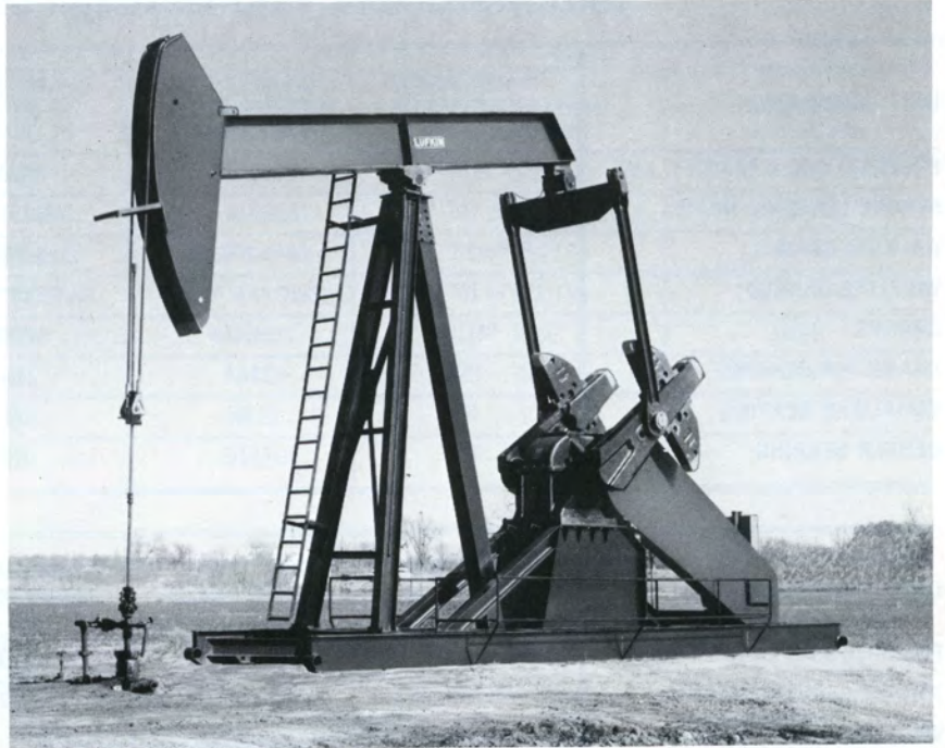
FIGURE 13 HEAVY DUTY PORTABLE "STRONGBACK" base is available for all units. Bases are also available with "Uniset" plated bottom to permit installation directly on soil with a minimum bearing capacity of 1500 pounds per square foot. Unit shown is a C-320D-256-120.
