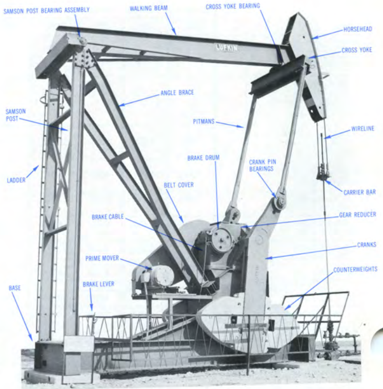
FIGURE 32 Mark II Pumping Unit
