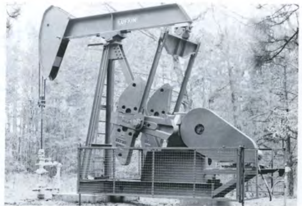
Two-point foundation reduces base stresses as well as installation costs and is easily transportable.
